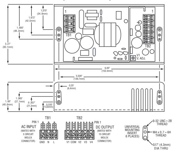
Figure-1 - Mechanical Drawing
