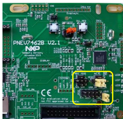
Fig 5. Host Interface selection – USB mode
