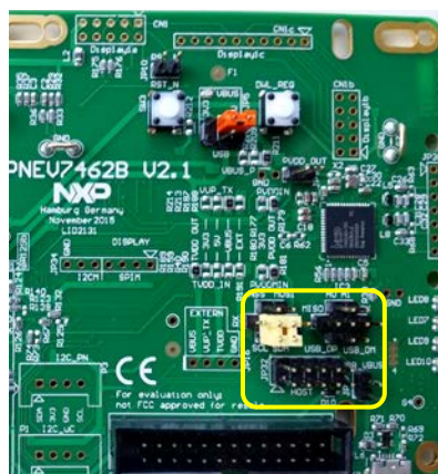
Fig 6. Host Interface selection - I2C mode
