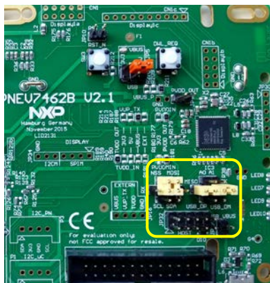
Fig 7. Host Interface selection - SPI
