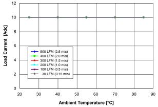
Fig. 1.5V.1: Available load current vs. ambient temperature and airflow rates for Vout = 1.5V converter mounted vertically with Vin = 12V, and maximum MOSFET temperature ≤ 120°C.
