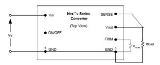
Fig. C: Configuration for programming output voltage.
