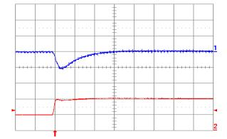
Fig. 1.0V.7: Output voltage response for Vout = 1.0V to positive load current step change from 5A to 10A with slew rate of 5A/μs at Vin = 12V. Top trace: output voltage (100mV/div.); Bottom trace: load current (5A/div.). Co = 100μF ceramic. Time scale: 20μs/div.
