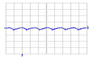
Fig. 2.0V.6: Output voltage ripple (20mV/div.) at full rated load current into a resistive load with external capacitance 100μF ceramic and Vin = 12V for Vout = 2.0V. Time scale: 2μs/div.
