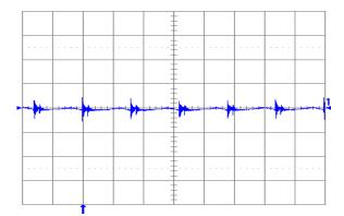
Fig. 1.2V.6: Output voltage ripple (20mV/div.) at full rated load current into a resistive load with external capacitance 100μF ceramic and Vin = 12V for Vout = 1.2V. Time scale: 2μs/div.
