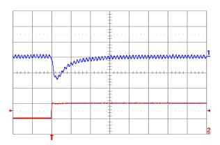
Fig. 5.0V.7: Output voltage response for Vout = 5.0V to positive load current step change from 5A to 10A with slew rate of 5A/μs at Vin = 12V. Top trace: output voltage (100mV/div.); Bottom trace: load current (5A/div.). Co = 100μF ceramic. Time scale: 20μs/div.
