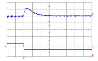
Fig. 1.5V.8: Output voltage response for Vout = 1.5V to negative load current step change from 10A to 5A with slew rate of -5A/µs at Vin = 12V. Top trace: output voltage (100mV/div.); Bottom trace: load current (5A/div.). Co = 100µF ceramic. Time scale: 20µs/div.
