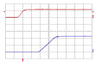
Fig. 1.2V.5: Turn-on transient for Vout = 1.2V with application of Vin at full rated load current (resistive) and 100μF external capacitance at Vin = 12V. Top trace: Vin (10V/div.); Bottom trace: output voltage (0.5V/div.); Time scale: 2ms/div.
