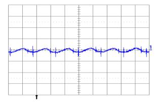
Fig. 2.5V.6: Output voltage ripple (20mV/div.) at full rated load current into a resistive load with external capacitance 100μF ceramic and Vin = 12V for Vout = 2.5V. Time scale: 2μs/div.
