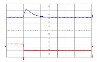
Fig. 2.0V.8: Output voltage response for Vout = 2.0V to negative load current step change from 10A to 5A with slew rate of -5A/µs at Vin = 12V. Top trace: output voltage (100mV/div.); Bottom trace: load current (5A/div.). Co = 100µF ceramic. Time scale: 20µs/div.
