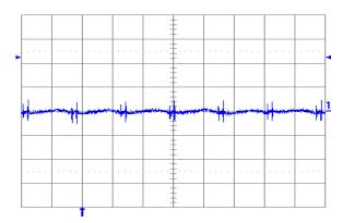
Fig. 1.0V.6: Output voltage ripple (20mV/div.) at full rated load current into a resistive load with external capacitance 100μF ceramic and Vin = 12V for Vout = 1.0V. Time scale: 2μs/div.
