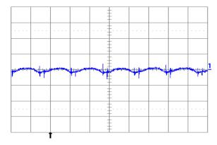
Fig. 1.5V.6: Output voltage ripple (20mV/div.) at full rated load current into a resistive load with external capacitance 100μF ceramic and Vin = 12V for Vout = 1.5V. Time scale: 2μs/div.
