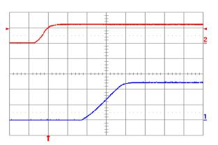
Fig. 2.5V.5: Turn-on transient for Vout = 2.5V with application of Vin at full rated load current (resistive) and 100µF external capacitance at Vin = 12V. Top trace: Vin (10V/div.); Bottom trace: output voltage (1V/div.); Time scale: 2ms/div.
