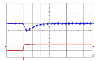
Fig. 1.8V.7: Output voltage response for Vout = 1.8V to positive load current step change from 5A to 10A with slew rate of 5A/μs at Vin = 12V. Top trace: output voltage (100mV/div.); Bottom trace: load current (5A/div.). Co = 100μF ceramic. Time scale: 20μs/div.
