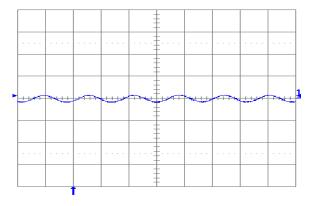
Fig. 1.8V.6: Output voltage ripple (20mV/div.) at full rated load current into a resistive load with external capacitance 100μF ceramic and Vin = 12V for Vout = 1.8V. Time scale: 2μs/div.
