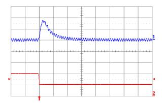
Fig. 5.0V.8: Output voltage response for Vout = 5.0V to negative load current step change from 10A to 5A with slew rate of -5A/µs at Vin = 12V. Top trace: output voltage (100mV/div.); Bottom trace: load current (5A/div.). Co = 100µF ceramic. Time scale: 20µs/div.
