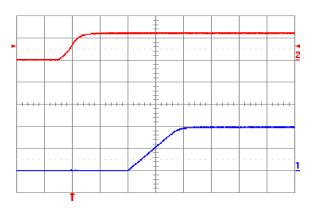
Fig. 1.0V.5: Turn-on transient for Vout = 1.0V with application of Vin at full rated load current (resistive) and 100μF external capacitance at Vin = 12V. Top trace: Vin (10V/div.); Bottom trace: output voltage (0.5V/div.); Time scale: 2ms/div.
