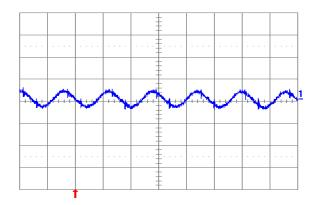
Fig. 3.3V.6: Output voltage ripple (20mV/div.) at full rated load current into a resistive load with external capacitance 100μF ceramic and Vin = 12V for Vout = 3.3V. Time scale: 2μs/div.
