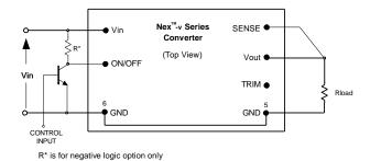
Fig. A: Circuit configuration for ON/OFF function.
