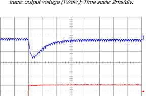
Fig. 3.3V.7: Output voltage response for Vout = 3.3V to positive load current step change from 5A to 10A with slew rate of 5A/μs at Vin = 12V. Top trace: output voltage (100mV/div.); Bottom trace: load current (5A/div.). Co = 100μF ceramic. Time scale: 20μs/div.
