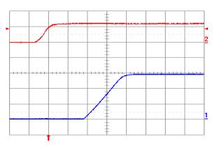
Fig. 1.5V.5: Turn-on transient for Vout = 1.5V with application of Vin at full rated load current (resistive) and 100µF external capacitance at Vin = 12V. Top trace: Vin (10V/div.); Bottom trace: output voltage (0.5V/div.); Time scale: 2ms/div.
