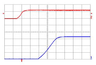
Fig. 3.3V.5: Turn-on transient for Vout = 3.3V with application of Vin at full rated load current (resistive) and 100μF external capacitance at Vin = 12V. Top trace: Vin (10V/div.); Bottom trace: output voltage (1V/div.); Time scale: 2ms/div.
