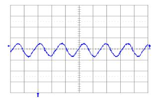
Fig. 5.0V.6: Output voltage ripple (20mV/div.) at full rated load current into a resistive load with external capacitance 100μF ceramic and Vin = 12V for Vout = 5.0V . Time scale: 2μs/div.
