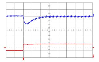
Fig. 1.5V.7: Output voltage response for Vout = 1.5V to positive load current step change from 5A to 10A with slew rate of 5A/μs at Vin = 12V. Top trace: output voltage (100mV/div.); Bottom trace: load current (5A/div.). Co = 100μF ceramic. Time scale: 20μs/div.
