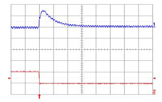
Fig. 3.3V.8: Output voltage response for Vout = 3.3V to negative load current step change from 10A to 5A with slew rate of -5A/µs at Vin = 12V. Top trace: output voltage (100mV/div.); Bottom trace: load current (5A/div.). Co = 100µF ceramic. Time scale: 20µs/div.
