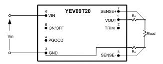
Figure 21. Remote Sense Circuit Configuration
