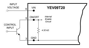
Figure 20. Circuit Configuration For ON/OFF Function
