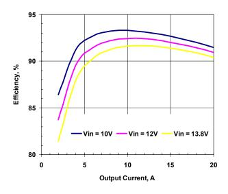
Figure 3. Efficiency vs. Load. Vout=2.5
