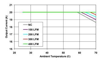
Figure 14. Derating Curves at Vo=1.2Vdc
