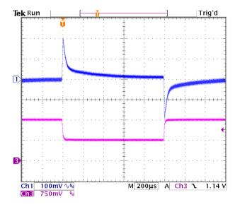
Figure 12. Transient Response to Dynamic Load Change from 50% to 100% of full load (Vin=12V, Vo=5.0Vdc). Ch3 – lout. Scale=10A/div
