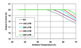
Figure 17. Derating Curves at Vo=3.3Vdc
