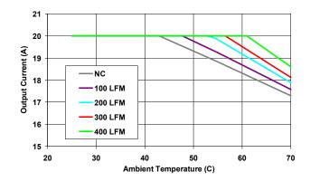
Figure 18. Derating Curves at Vo=5.0Vdc
