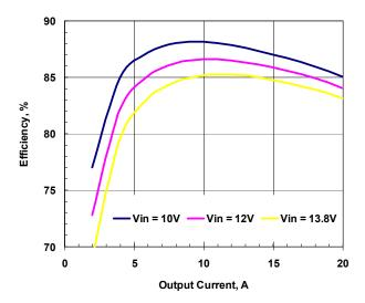
Figure 2. Efficiency vs. Load. Vout=1.2V
