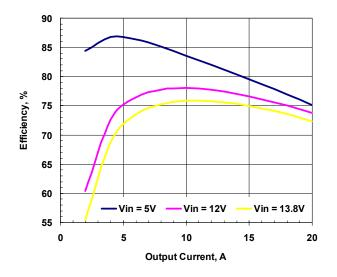
Figure 1. Efficiency vs. Load. Vout=0.6V
