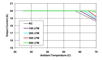
Figure 15. Derating Curves at Vo=1.8Vdc
