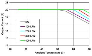
Figure 16. Derating Curves at Vo=2.5Vdc
