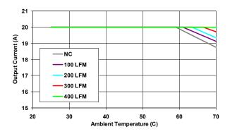
Figure 13. Derating Curves at Vo=0.9Vdc
