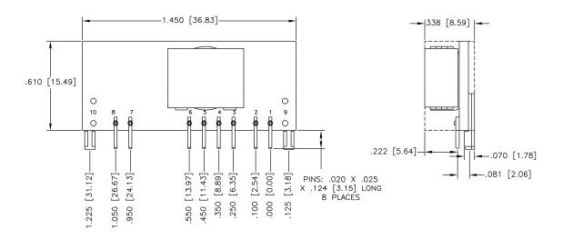
Figure 23. Mechanical Drawing
