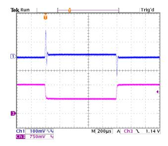
Figure 10. Transient Response to Dynamic Load Change from 50% to 100% of full load (Vin=12V, Vo=0.6Vdc). Ch3 – lout. Scale=10A/div
