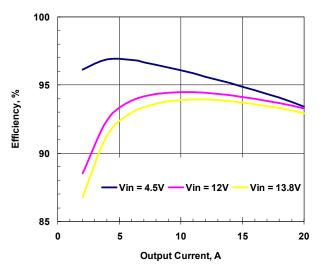
Figure 4. Efficiency vs. Load. Vout=3.3V
