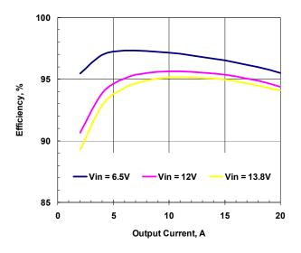
Figure 5. Efficiency vs. Load. Vout=5.0V
