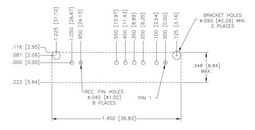
Figure 24. Recommended Footprint - Top View
