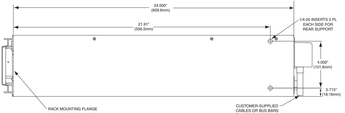
This kit is used to cover an unused right-side slot of the FRH7000 Power Shelf (as viewed from the front of the FRH7000). The kit can be installed before, or after installation of the power shelf into the rack.
