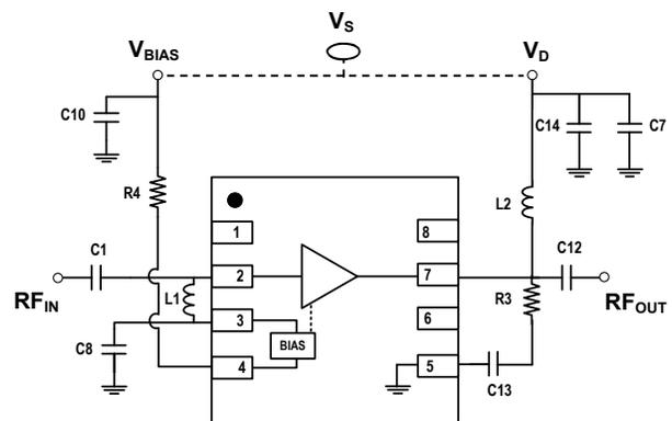
Optional schematic illustrates alternate grounding choice for  $C13$  through pin 5. Pin 5 is grounded internally in the package. Electrical performance of both layout methods is identical.
