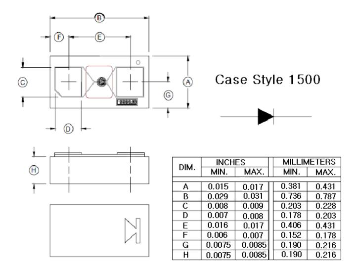
1. Pad finish is .2 microns of gold over 4 microns of nickel.
