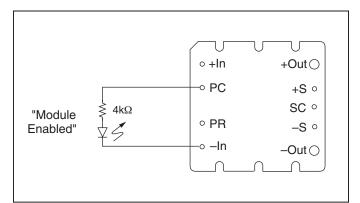
**Figure 4** — LED on-state indicator.
