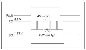
*Figure 5* — PC/SC module alarm timing.
