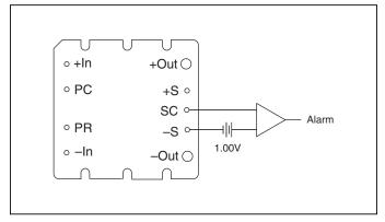
Figure 7 — Secondary side on-state indicator.
