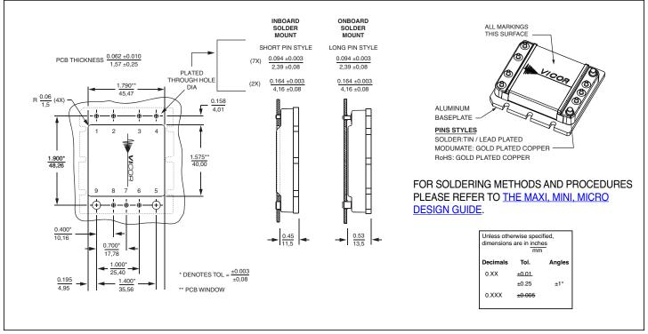
Figure 13 — PCB mounting specifications
