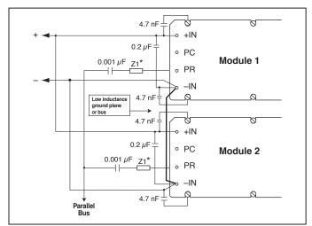
Figure 9 — AC coupled single-wire interface.
