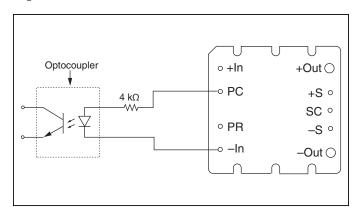
Figure 6 — Isolated on-state indicator.
