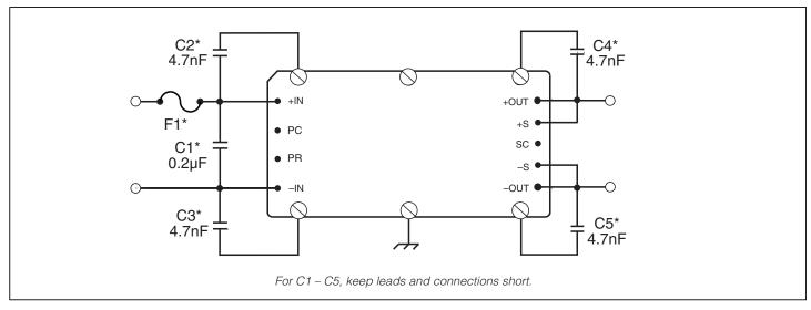
**Figure 1** — Basic module operation requires fusing, grounding, bypassing capacitors.
