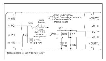
*Figure 3* — PC/SC module alarm logic.
