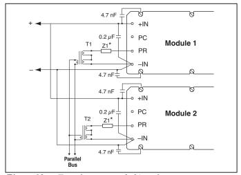
Figure 10 — Transformer-coupled interface.
