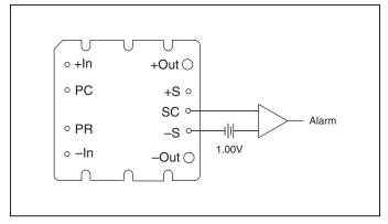
*Figure* 7 — *Secondary side on-state indicator.*
