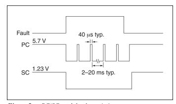
**Figure 5** — PC/SC module alarm timing.
