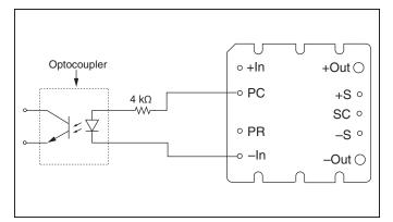
Figure 6 — Isolated on-state indicator.
