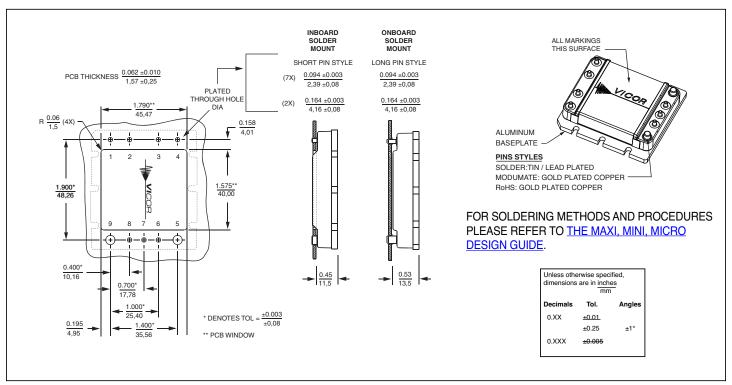
Figure 13 — PCB mounting specifications
