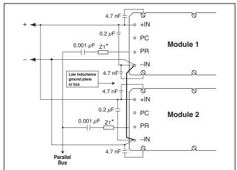
Figure 9 — AC coupled single-wire interface.
