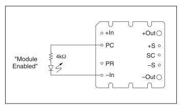
**Figure 4** — LED on-state indicator.
