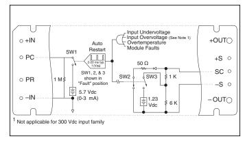
*Figure 3* — PC/SC module alarm logic.
