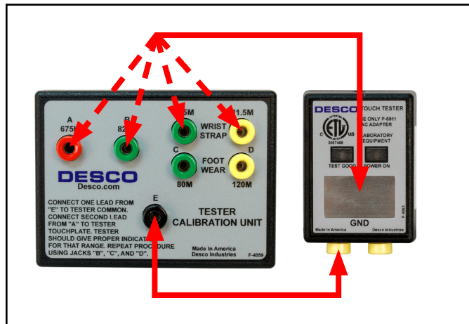
Figure 9. Verifying the calibration of the Wrist Strap Touch Tester
