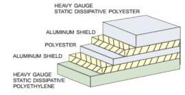
SCS Moisture Barrier Bags are packaged in a polyethylene bag.
