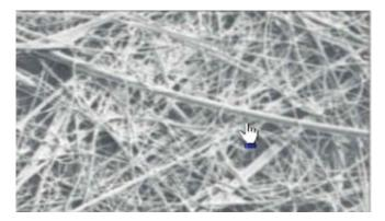
Photomicrograph of the fiber weave of a 3M filter (500x)
