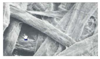
Photomicrograph of the fiber weave of a conventional filter bag (500x)
