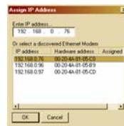
If the Ethernet RF Modem is left in DHCP mode, it may become necessary to reconfigure a mapped com port any time an IP address is re-assigned by the DHCP server. Dynamic addressing is supported, but setting a static IP address can simplify the application.
