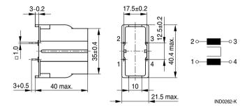
Tolerances to ISO 2768-C unless otherwise noted. Dimensions in mm.
