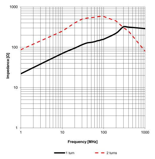
GENERAL TOLERANCE CREATED CHECKED Würth Elektronik eiSos GmbH & Co. KG EMC & Inductive Solutions DaMa SMu DIN ISO 2768-1m Max-Eyth-Str. 1 74638 Waldenburg **WE-AFB EMI Suppression Axial** Tel. +49 (0) 79 42 945 - 0 **Ferrite Bead** ORDER CODE www.we-online.com 74270095 eiSos@we-online.com REVISION STATUS BUSINESS UNIT PAGE Valid 006.000 2016-08-01 eiSos 2/4
