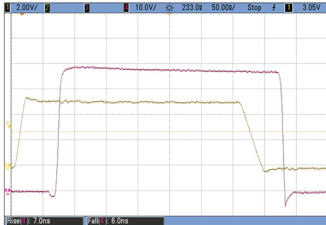
Figure 4: Typical Waveforms for  $V_{IN} = 48$  V to 5 V/35 A (300 kHz) Buck converter
