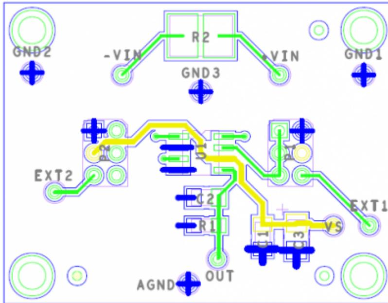
Figure 4. Component Side Layout
