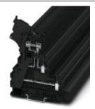
Fuse modular terminal block, Connection method: Screw connection, Cross section:  $0.14 \text{ mm}^2$ -  $4 \text{ mm}^2$ , AWG: 26 - 10, Nominal current: 30 A, Nominal voltage: 60 V, Width: 6.2 mm, Fuse type: G / 5 x 20, Fuse type: Glass / ceramics / ..., Mounting type: NS 35/7.5, NS 35/15, Color: black
