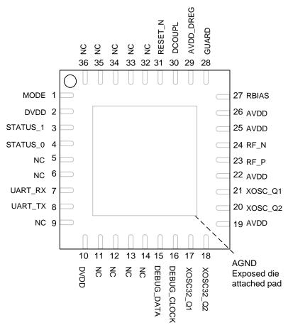
Figure 1: Pinout top view
