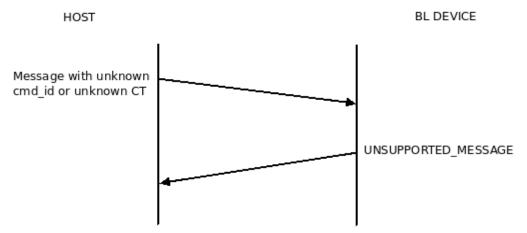
Figure 4. Unsupported data received by BL Device
