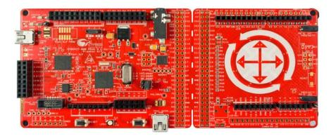
The  $PSoC^{\otimes}$  4 L-Series Pioneer Kit is a low-cost hardware and software platform to enable design and debug of the PSoC 4200L device.
