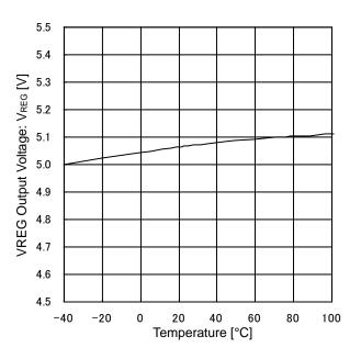
Figure 9. VREG Output Voltage vs Temperature
