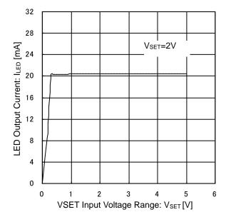
Figure 6. LED Output Current vs VSET Input Voltage Range (VLED Dependency of ILED)
