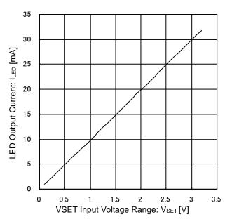
Figure 5. LED Output Current vs VSET Input Voltage Range (VSET Constant electric current Characteristics) (Unless specified, V<sub>CC</sub>=24V, Ta=25°C)
