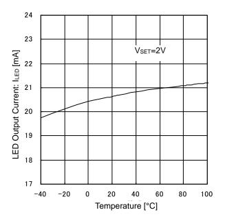
Figure 7. LED Output Current vs Temperature (Constant Electric Current Temperature Characteristic)
