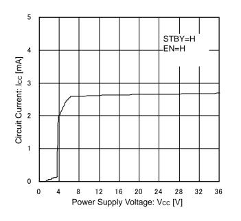
Figure 4. Circuit Current vs Power Supply Voltage (Operating Mode)
