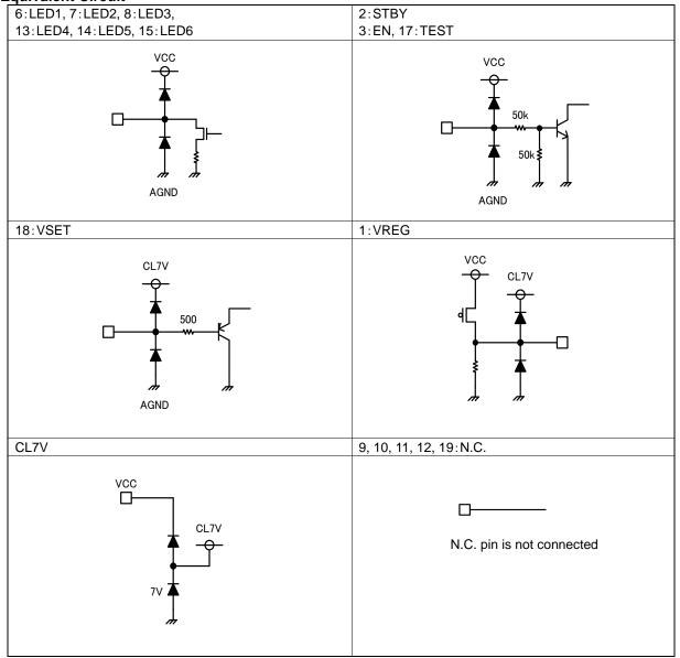
Note: The voltage clamp element of 7V is connected to CL7V.
