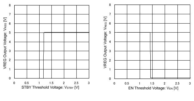
Figure 10. VREG Output Voltage vs STBY Threshold Voltage
