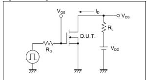
Fig.2-1 Gate Charge Measurement Circuit
