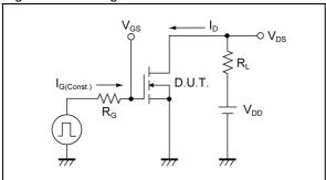
Fig.3-1 Avalanche Measurement Circuit
