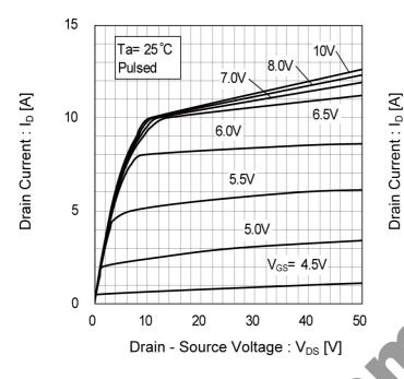
Fig.6 Typical Output Characteristics(II)
