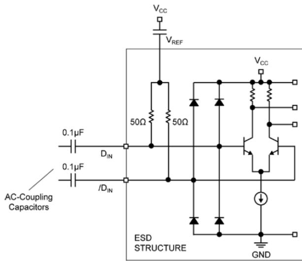
Figure 2. Input Structure
