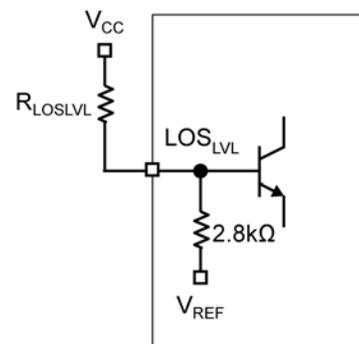
Figure 5. LOS<sub>LVL</sub> Setting Circuit
