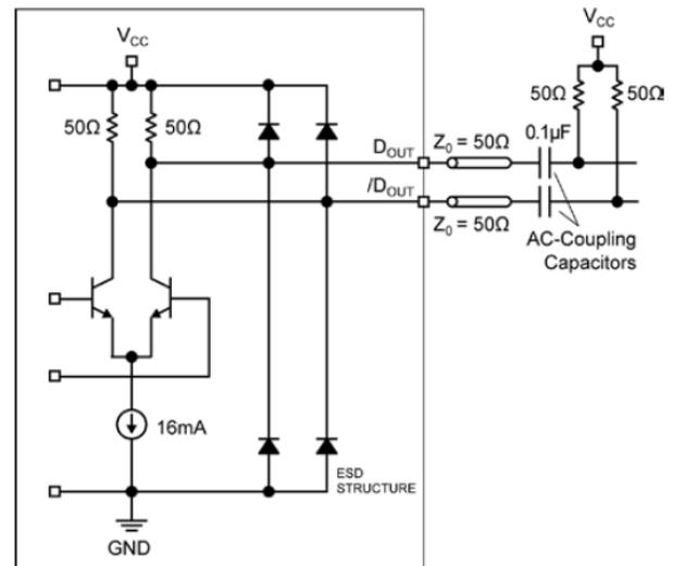
Figure 3. Output Structure
