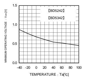
Fig.12 Operating Limit Voltage
