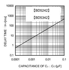
Fig.14 Delay Time ( $t_{\text{PLH}}$ ) and  $C_{\text{T}}$  Terminal External Capacitance
