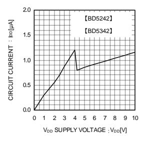
Fig.3 Circuit Current
