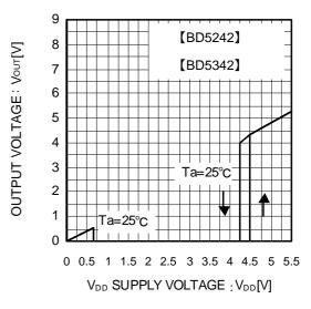
Fig.6 I/O Characteristics
