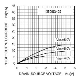
Fig.5 "High" Output Current
