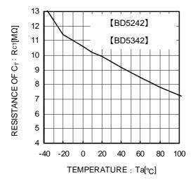
Fig.13 C<sub>T</sub> Terminal Circuit Resistance
