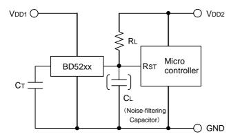
Fig.18 Open Drain Output Type
