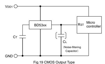
Application examples of BD52xx series (Open Drain output type) and BD53xx series (CMOS output type) are shown below.
