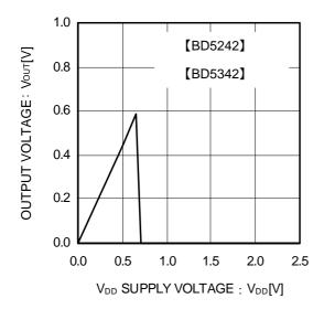
Fig.7 Operating Limit Voltage
