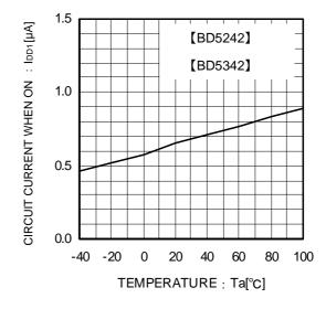
Fig.10 Circuit Current when ON
