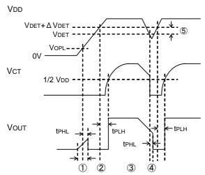
Fig.17 Timing Waveform
