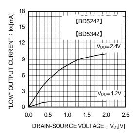
Fig.4 "Low" Output Current
