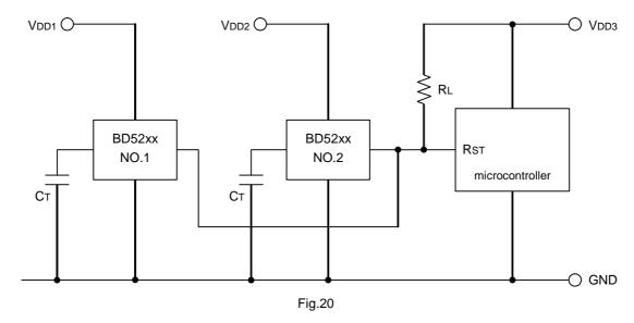
To reset the microcontroller when many independent power supplies are used in the system, OR connect an open drain output type (BD52xx series) to the microcontroller's input with pull-up resistor to the supply voltage of the microcontroller (V<sub>DD3</sub>) as shown in Fig. 20. By pulling-up to V<sub>DD3</sub>, output "High" voltage of micro-controller power supply is possible.
