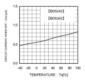
Fig.11 Circuit Current when OFF
