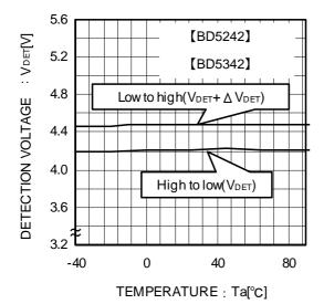
Fig.9 Detection Voltage Release Voltage
