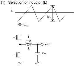
The inductance significantly depends on output ripple current. As seen in equation (1), the ripple current decreases as the inductor and/or switching frequency increases.
