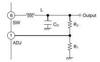
Figure 102. Determination of Output Voltage
