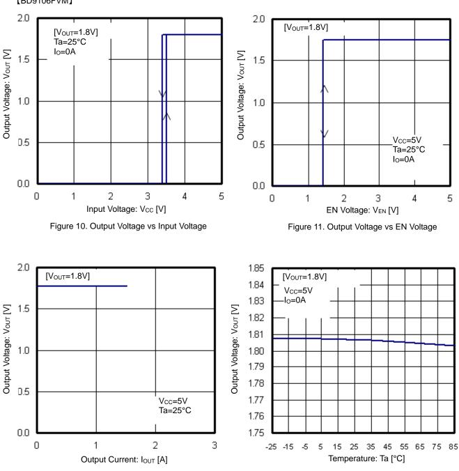
Figure 12. Output Voltage vs Output Current
