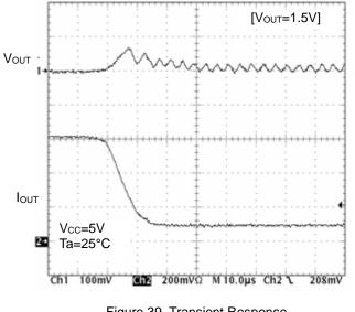
Figure 39. Transient Response (Io=600mA to 100mA, 10µs)
