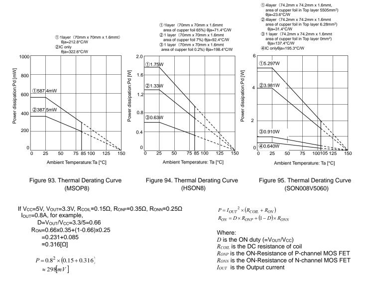
Since RONP is greater than RONN in these ICs, the dissipation increases as the ON duty becomes greater. Taking into consideration the dissipation shown above, thermal design must be carried out with allowable sufficient margin.
