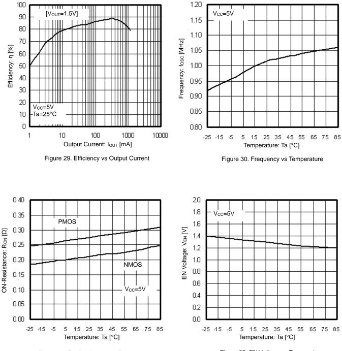
Figure 31. ON-Resistance vs Temperature
