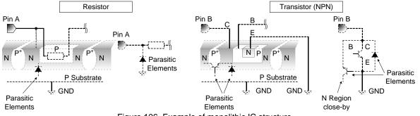
Figure 106. Example of monolithic IC structure
