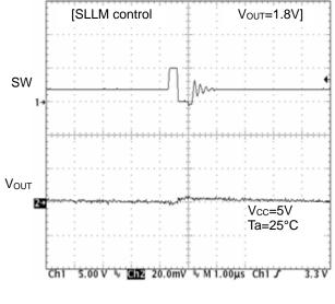
Figure 21. SW Waveform (Io=10mA)
