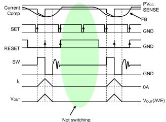
Figure 87. SLLM Switching Timing Chart
