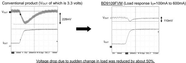
Figure 90. Comparison of Transient Response
