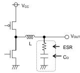
Figure 97. Output Capacitor
