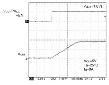
Figure 20. Soft Start Waveform
