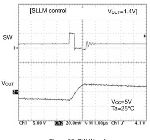
Figure 66. SW Waveform ( Io=10mA)
