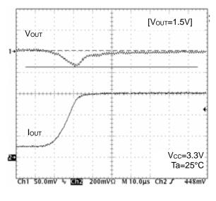
Figure 83. Transient Response (Io=100mA to 600mA, 10µs)
