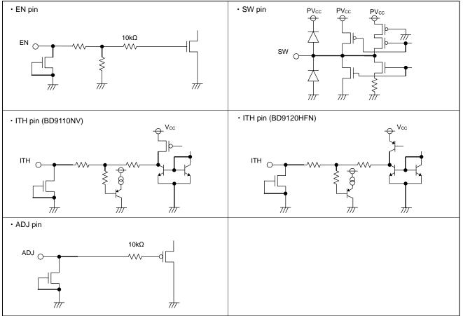
Figure 105. I/O Equivalent Circuit
