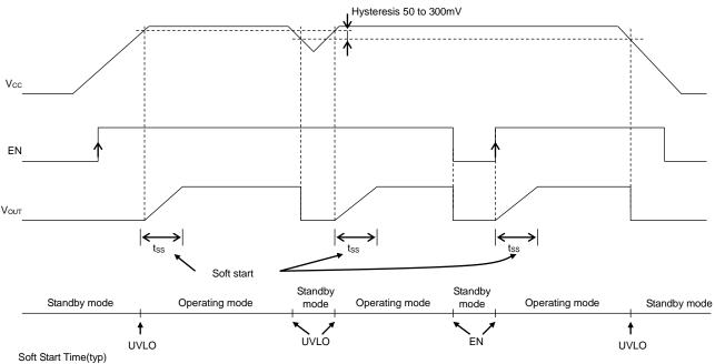
Figure 88. Soft Start, Shutdown, UVLO Timing Chart
