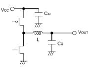
Figure 98. Input Capacitor
