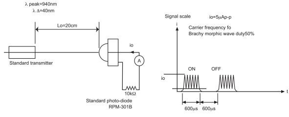
Fig.2 Measurement of standard transmitter proofreading
