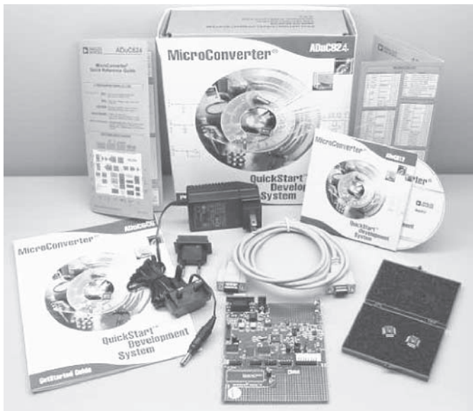
Figure 67. Components of the QuickStart Development System
