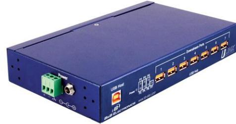
The UHR207 and UHR307 are **Industrial Grade Seven Port USB Hubs**. Model UHR307 includes 4 kV isolation. They are designed and tested to meet heavy industrial EMC standards. High retention USB connectors hold standard USB cables tight and are perfect for high vibration applications – requiring up to 3.2 lbs-force to disconnect them.
