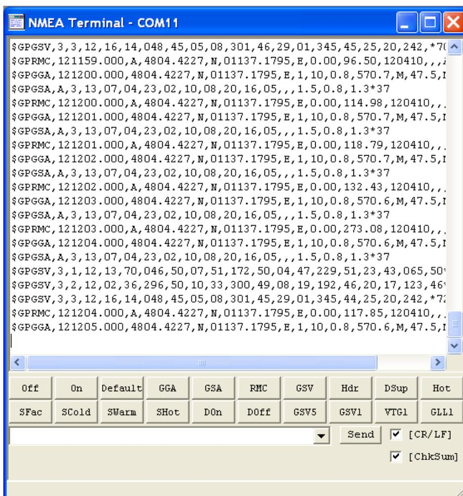
Figure 7: GPS Cockpit NMEA terminal with NMEA data
