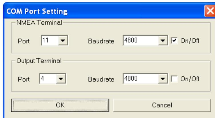
Figure 6: GPS Cockpit COM Port Setting window
