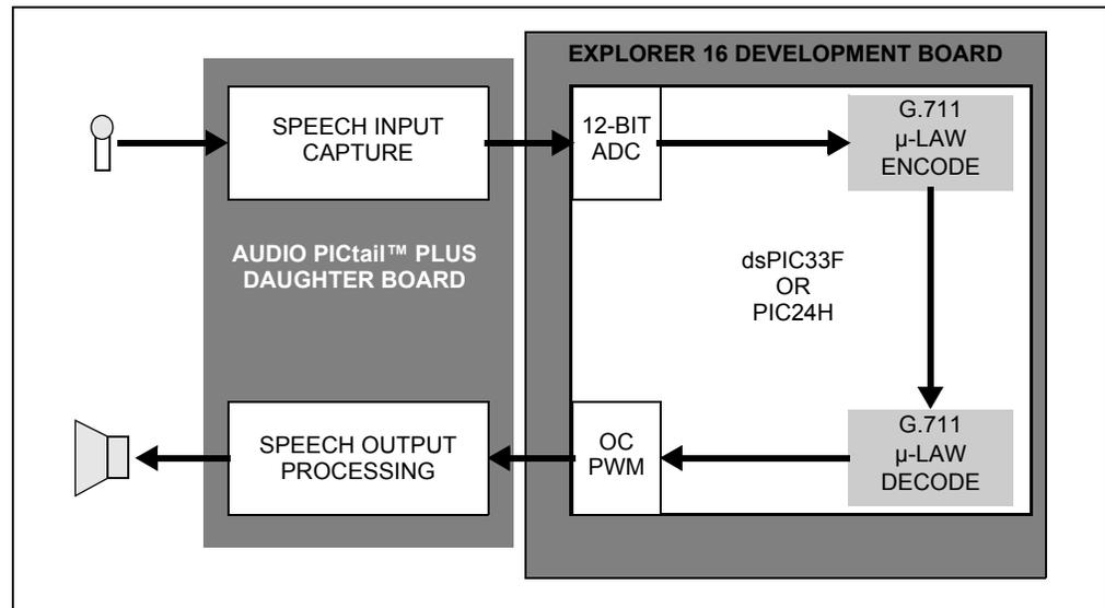
The Audio PICtail Plus Daughter Board then processes the PWM signal through the PWM filter to produce an analog audio signal. This signal is amplified and output through the speaker.
