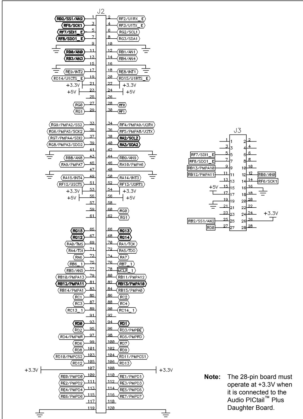
**Note:** The 28-pin board must operate at +3.3V when it is connected to the Audio PICtail™ Plus Daughter Board.
