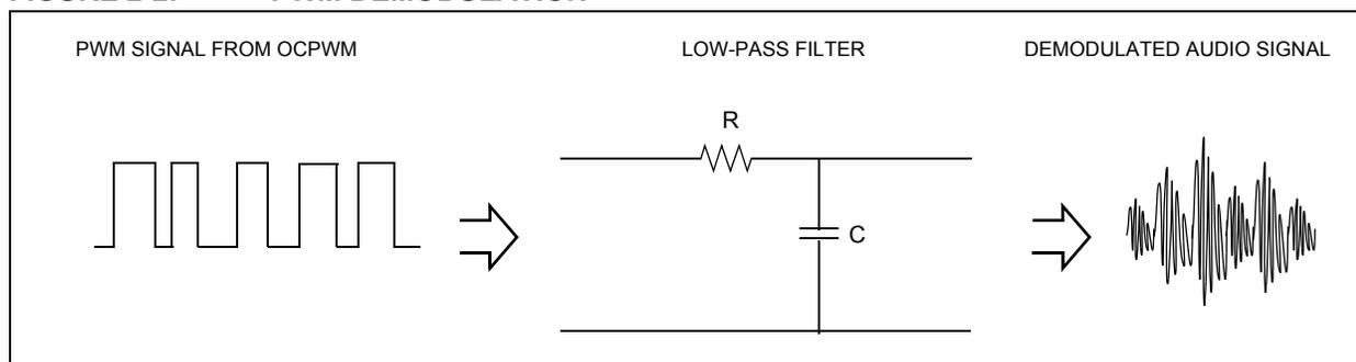
The output of the low-pass filter feeds both the Line Output and Headphone amplifiers (through Output Select Jumper J4). The Line Output amplifier drives external audio recording equipment or an external audio power amplifier. The amplifier is an AC inverting amplifier with adjustable gain. The gain can be adjusted to match the input level requirements of the external audio equipment, and can be varied from -1 dB to 10 dB.
