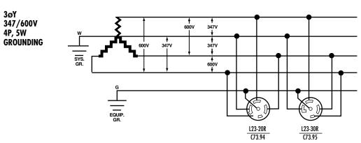
Most Woodhead plugs, connectors, and receptacles are standard NEMA configurations. As such, standard terminal identification is used to incorporate these devices in the wiring system.
