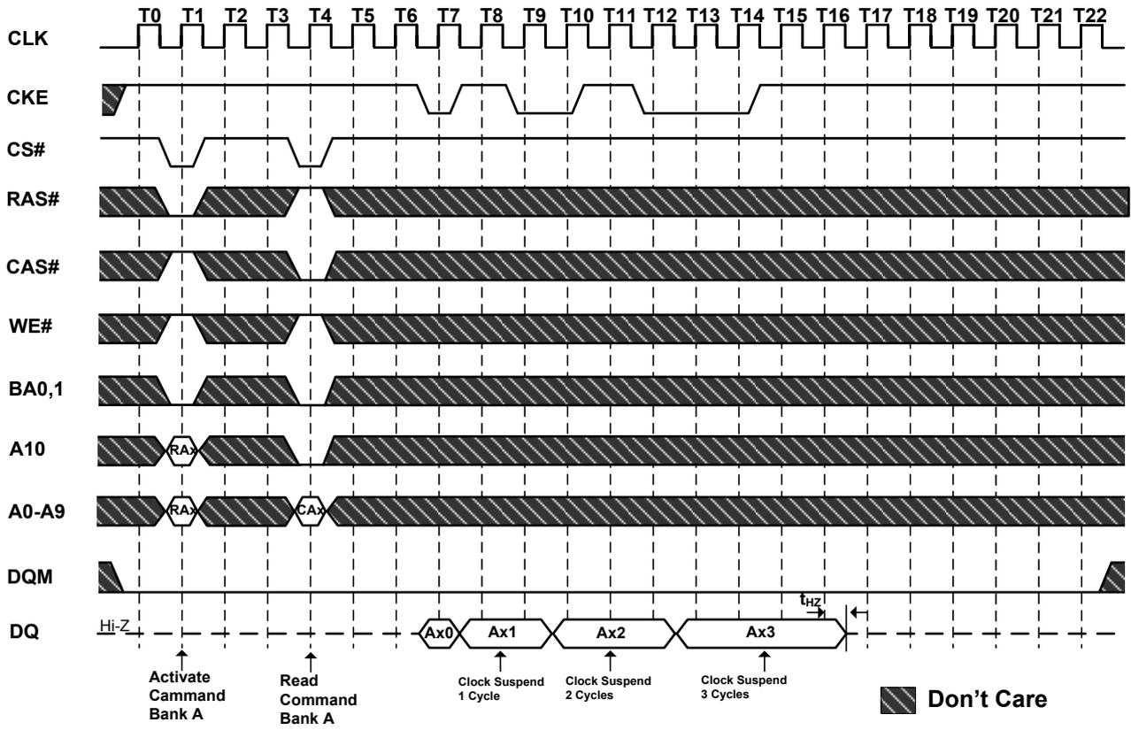
**Figure 25. Clock Suspension During Burst Write (Using CKE)**
