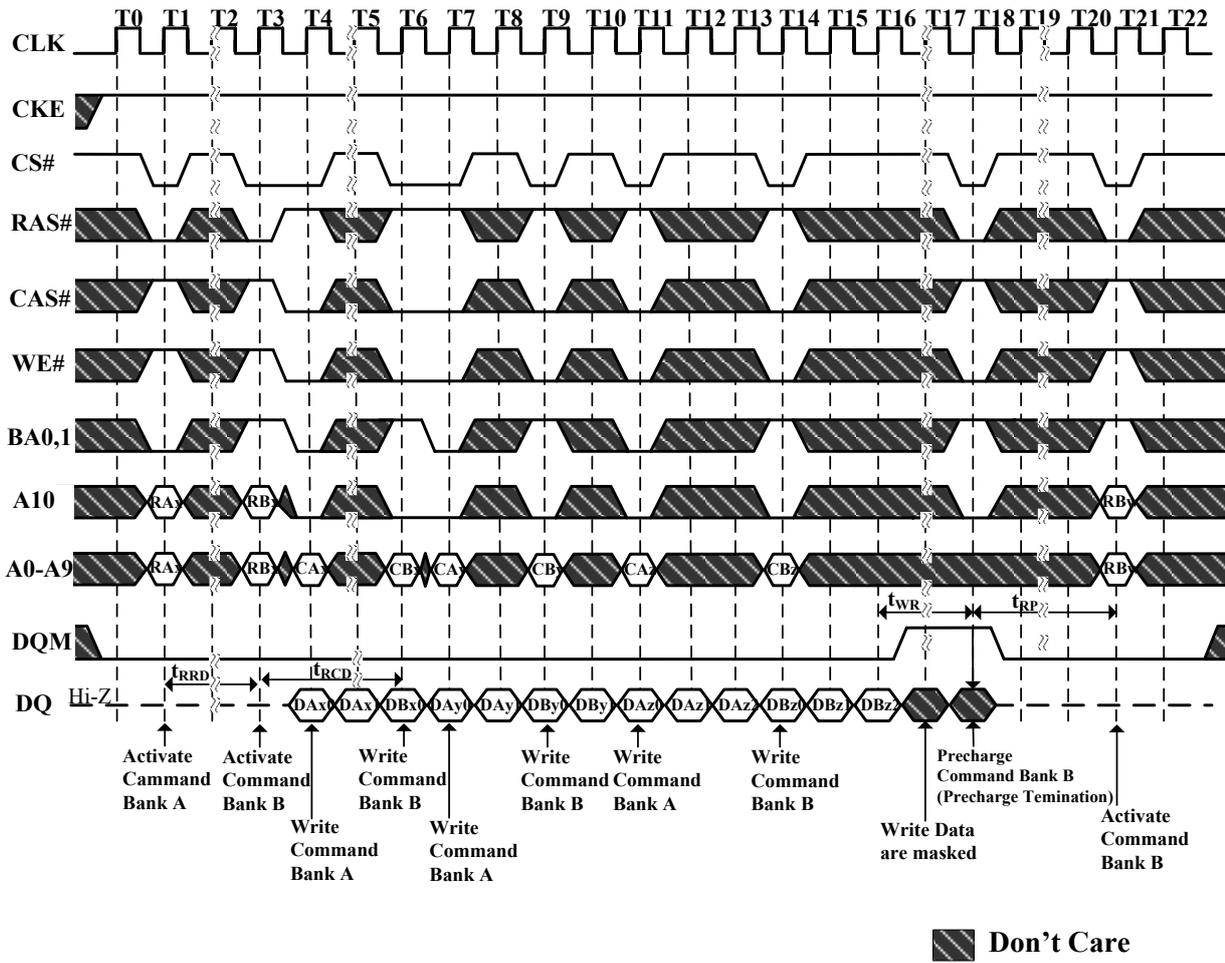
**Figure 42. Precharge Termination of a Burst**
