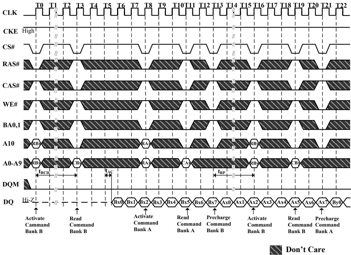
**Figure 30. Random Row Write (Interleaving Banks)**
