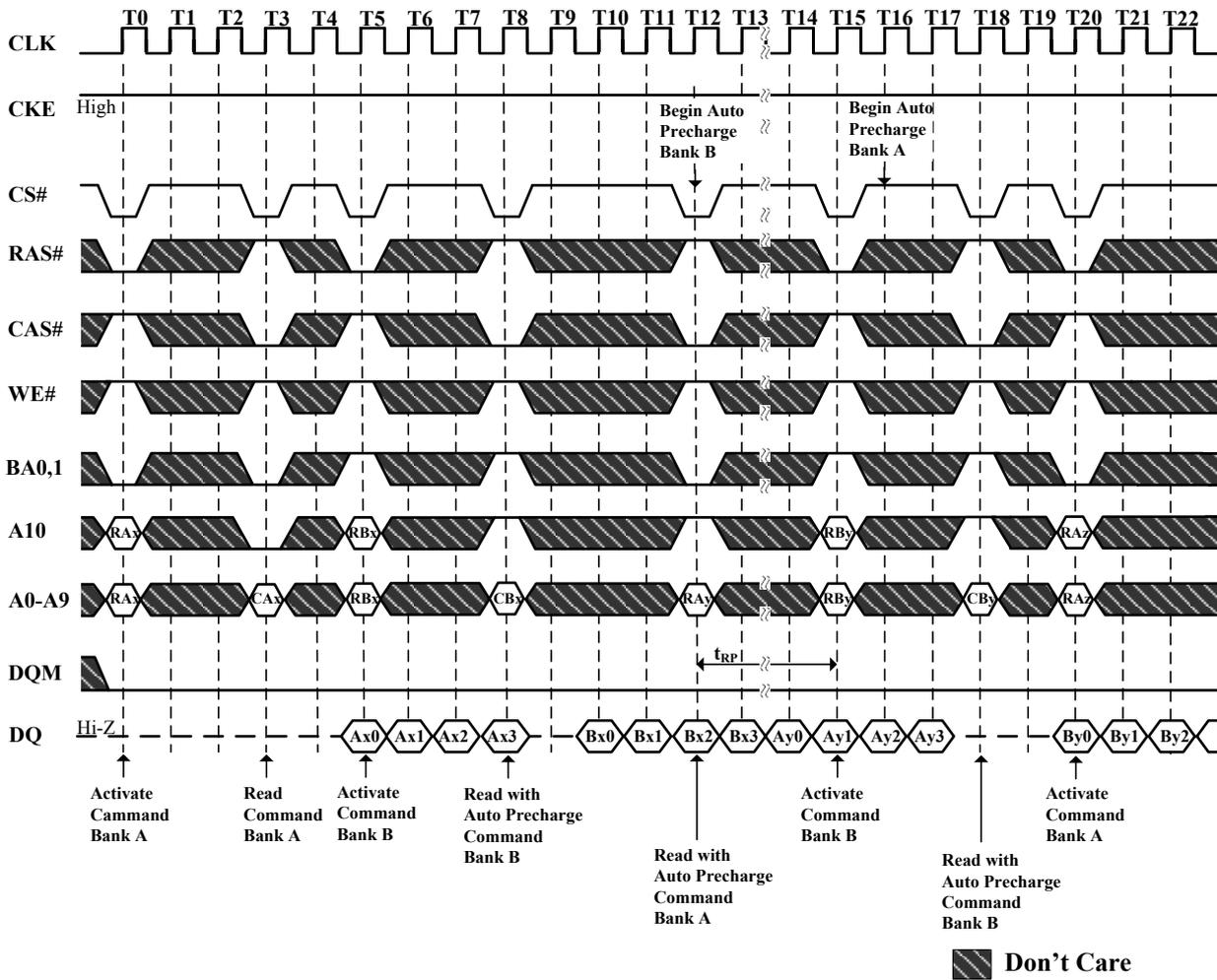
**Figure 34.2. Auto Precharge after Read Burst (Burst Length=4, CAS# Latency=3)**
