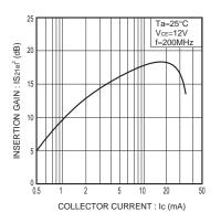
Fig.7 Insertion gain vs. collector current
