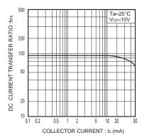
Fig.1 DC current gain vs. collector current
