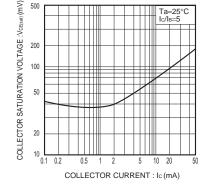
Fig.2 Collector-emitter saturation voltage vs. collector current
