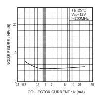
Fig.9 Noise factor vs. collector current
