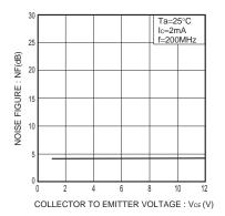
Fig.10 Noise factor vs. collector voltage
