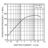
Fig.4 Gain bandwidth product vs. emitter current
