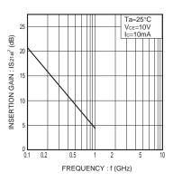
Fig.6 Insertion gain vs. frequency
