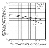
Fig.3 Capacitance vs. reverse bias voltage
