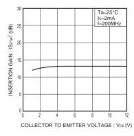
Fig.8 Insertion gain vs. collector voltage
