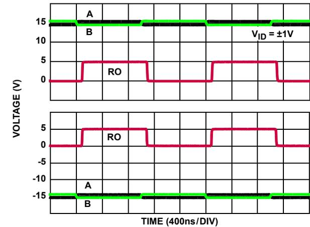
FIGURE 23. RECEIVER PERFORMANCE WITH  $\pm 15V$  CMV (ISL32475E)
