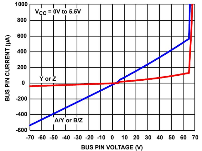
FIGURE 15. BUS PIN CURRENT vs BUS PIN VOLTAGE
