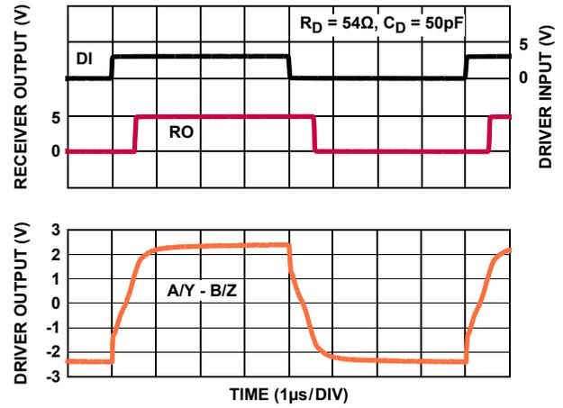
FIGURE 25. DRIVER AND RECEIVER WAVEFORMS (ISL32470E, ISL32472E)
