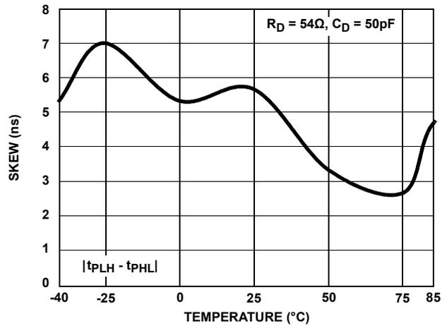
FIGURE 17. DRIVER DIFFERENTIAL SKEW vs TEMPERATURE (ISL32470E, ISL32472E)
