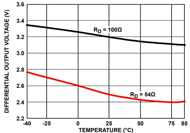
FIGURE 11. DRIVER DIFFERENTIAL OUTPUT VOLTAGE vs TEMPERATURE
