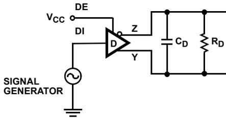
FIGURE 4A. TEST CIRCUIT
