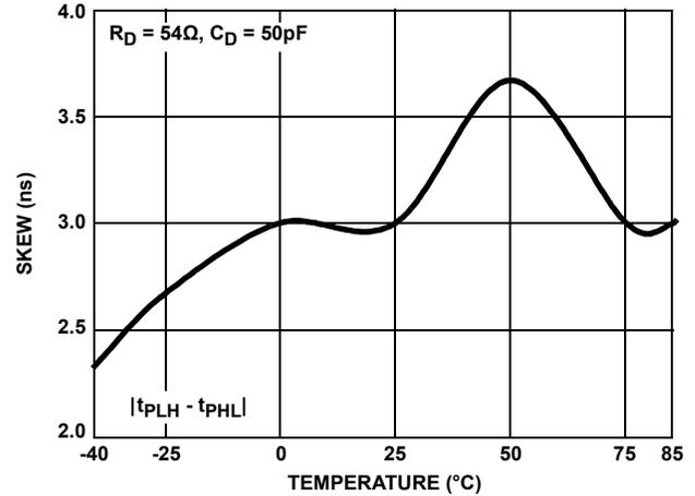
FIGURE 19. DRIVER DIFFERENTIAL SKEW vs TEMPERATURE (ISL32475E)
