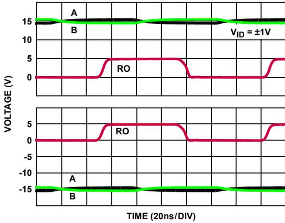
FIGURE 24. RECEIVER PERFORMANCE WITH  $\pm 15V$  CMV (ISL32478E)
