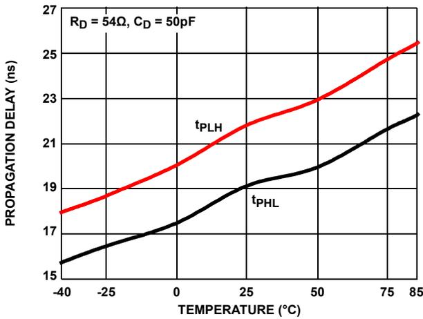
FIGURE 20. DRIVER DIFFERENTIAL PROPAGATION DELAY vs TEMPERATURE (ISL32478E)
