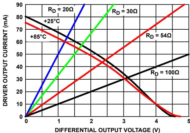
FIGURE 10. DRIVER OUTPUT CURRENT vs DIFFERENTIAL OUTPUT VOLTAGE
