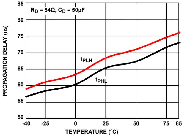
FIGURE 18. DRIVER DIFFERENTIAL PROPAGATION DELAY vs TEMPERATURE (ISL32475E)
