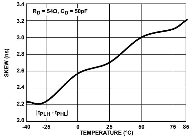
FIGURE 21. DRIVER DIFFERENTIAL SKEW vs TEMPERATURE (ISL32478E)
