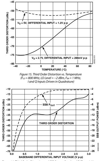
Figure 16. Third Order Distortion and SSB  $P_{OUT}$  vs. Baseband Differential Input Voltage ( $T_A = 25^{\circ}$ C,  $F_{LO} = 800$  MHz, LO Level = -2 dBm,  $F_{BB} = 1$  MHz,  $V_S = 2.7$  V)
