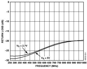
Figure 20. Return Loss (S22) of VOUT Output ( $T_A = 25^{\circ}$ C)
