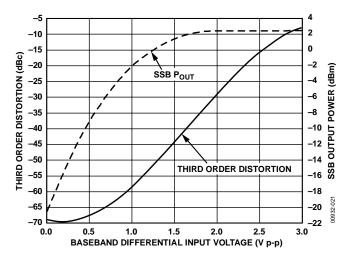
Figure 17. Third Order Distortion and SSB  $P_{OUT}$  vs. Baseband Differential Input Voltage ( $T_A = 25^{\circ}$ C,  $F_{LO} = 800$  MHz, LO Level = -2 dBm,  $F_{BB} = 1$  MHz,  $V_S = 5$  V)
