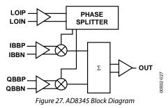
The LO interface generates two LO signals at 90° of phase difference with each other, to drive two mixers in quadrature. Baseband signals are converted into current form in the differential V-to-I converters, feeding into the two mixers. The outputs of the mixers are combined to feed the differential-to-single-ended converter, which provides a 50  $\Omega$  output interface. Bias currents to each section are controlled by the enable (ENBL) signal. A detailed description of each section follows.
