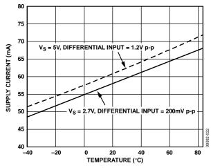
Figure 18. Power Supply Current vs. Temperature
