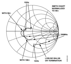
Figure 19. Smith Chart of LOIN Port S11 (LOIP Pin AC-Coupled to Ground); Curves with Balun and External Termination Resistors Also Shown  $(V_S = 5 V, T_A = 25^{\circ}C)$
