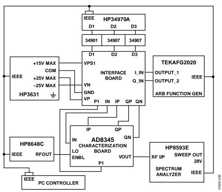
Figure 37. Characterization Board SSB Test Setup
