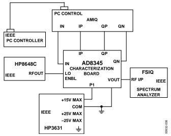
Figure 38. Test Setup for Evaluating AD8345 with Modulated Waveforms
