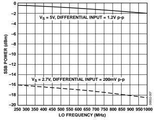
Figure 3. Single Sideband (SSB) Output Power ( $P_{OUT}$ ) vs. LO Frequency ( $F_{LO}$ ) (l and Q Inputs Driven in Quadrature at Baseband Frequency ( $F_{BB}$ ) = 1 MHz;  $T_A = 25 \,^{\circ}\text{C}$ )
