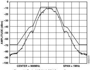
Figure 41. Typical AD8345 GSM Output Spectrum
