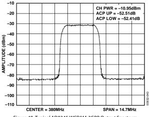
Figure 40. Typical AD8345 WCDMA 3GPP Output Spectrum
