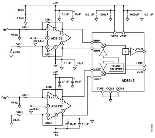
Figure 30. Single-Ended 1Q Drive Circuit
