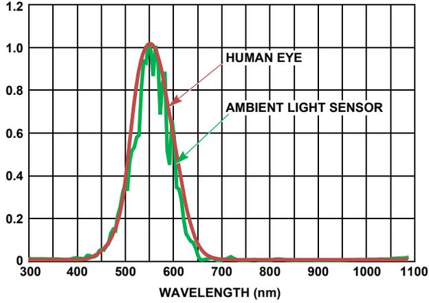
FIGURE 6. NORMALIZED SPECTRAL RESPONSE FOR AMBIENT LIGHT SENSING
