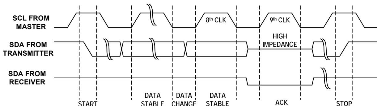
FIGURE 12. START, DATA STABLE, ACKNOWLEDGE AND STOP CONDITION
