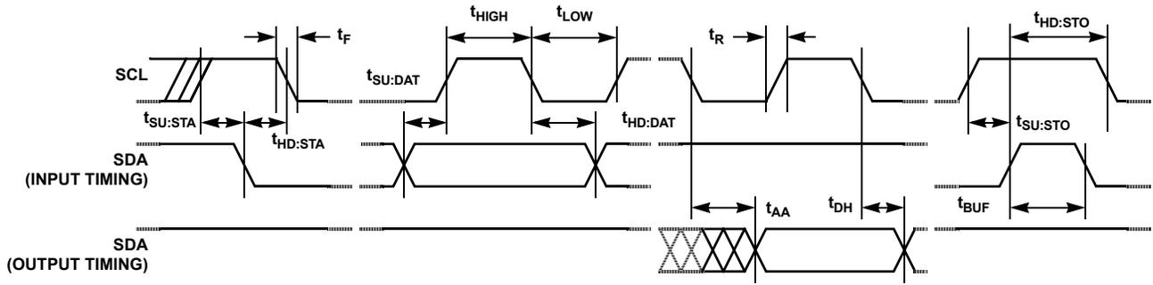
FIGURE 4. I<sup>2</sup>C BUS TIMING
