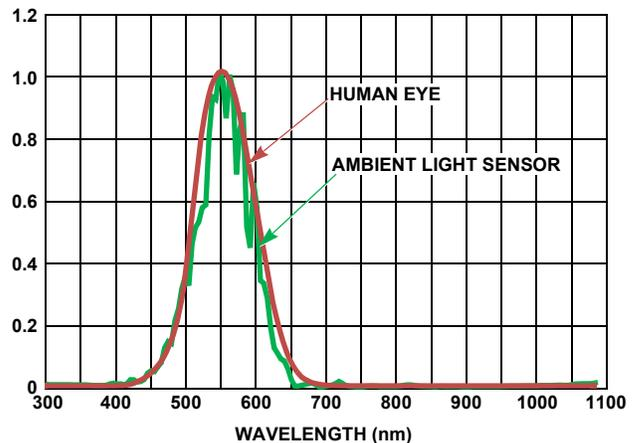
FIGURE 2. NORMALIZED SPECTRAL RESPONSE FOR AMBIENT LIGHT SENSING
