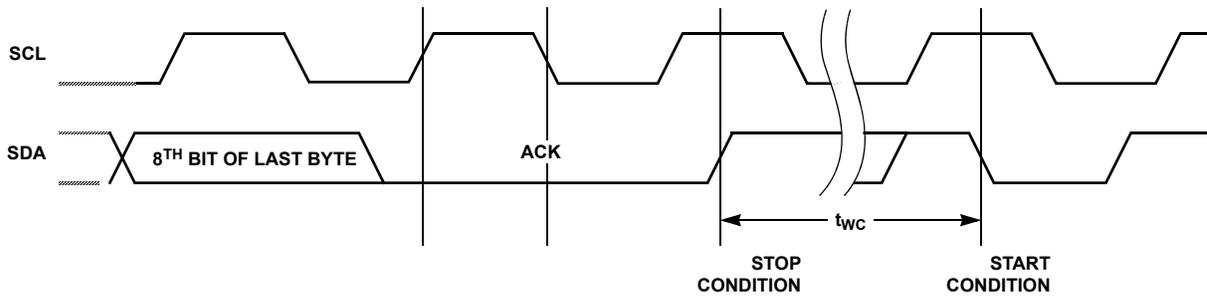
FIGURE 5. I<sup>2</sup>C WRITE CYCLE TIMING
