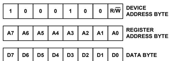
FIGURE 10. DEVICE ADDRESS, REGISTER ADDRESS AND DATA BYTE
