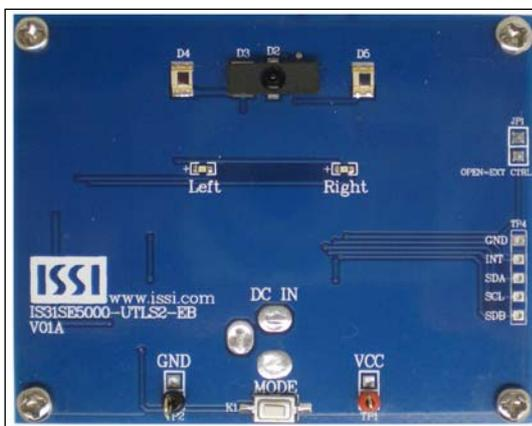
Figure 1: Photo of IS31SE5000 Evaluation Board
