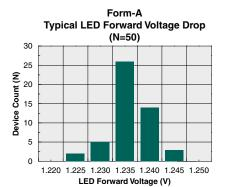
Form-A Typical LED Forward Voltage Drop
