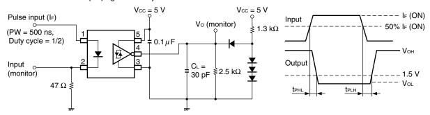
C∟ includes probe and stray wiring capacitance.
