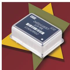
These unique OCXO / VCOCXO oscillator products provide temperature stabilities in the range of  $\pm 3$  ppb to  $\pm 25$  ppb, over the commercial, extended commercial or the industrial temperature range. Power requirements are 3W over the commercial temperature range and 4.5W over the industrial temperature range. Additionally, excellent aging is achieved through the use of overtone SC cut crystals.
