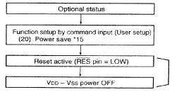
Set the time (tL) from reset active to turning off the VDD - Vss power (VDD - Vss = 1.8 V) longer than the time (th) when the potential of V5 ~ V1 becomes below the threshold voltage (approximately 1 V) of the LCD panel. For th, refer to the <Reference Data> of this event. When the is too long, insert a resistor between Vs and Vpp to reduce it.
