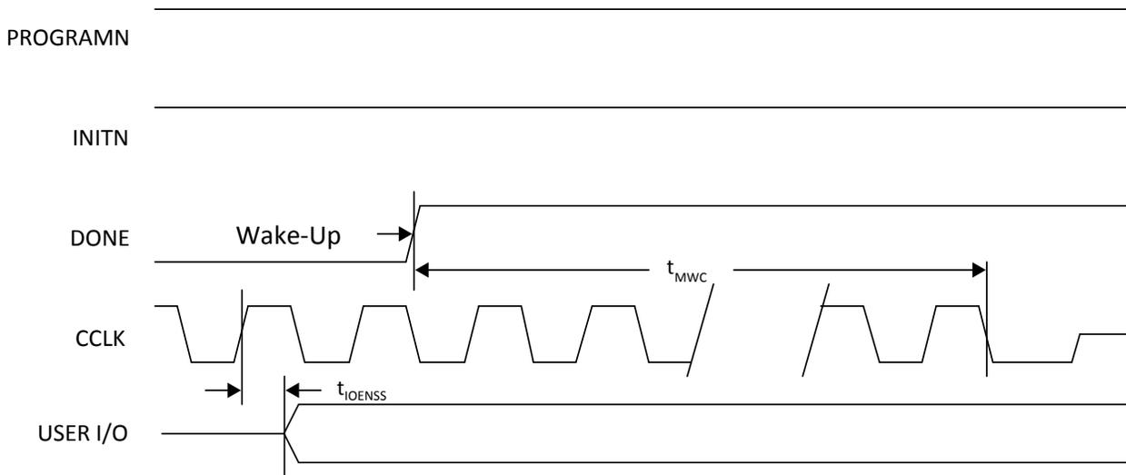
**Figure 3.21. Wake-Up Timing**
