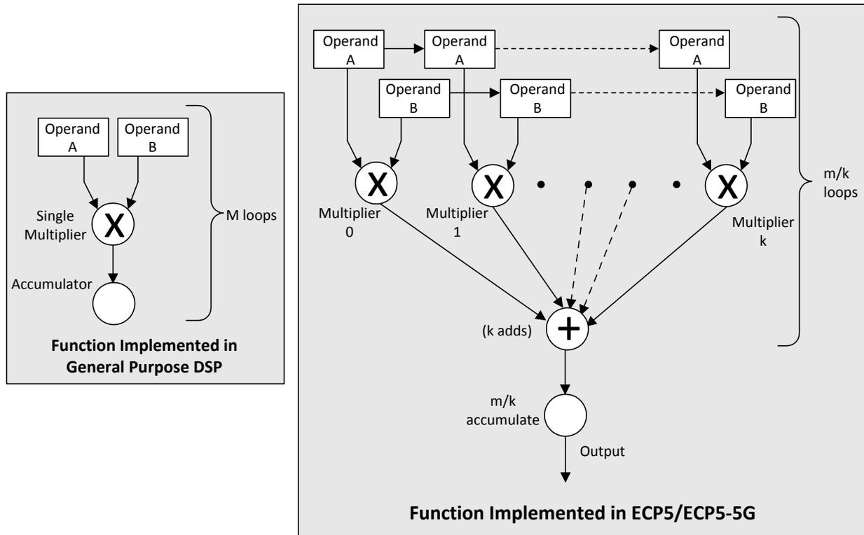
Figure 2.13. Comparison of General DSP and ECP5/ECP5-5G Approaches
