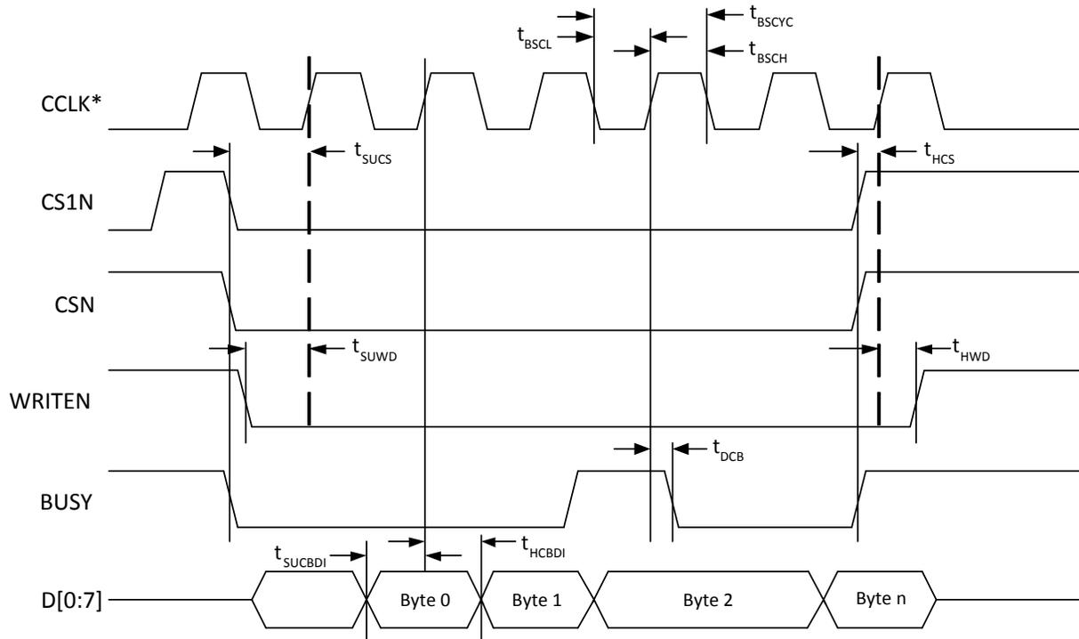
\*In Master Parallel Mode the FPGA provides CCLK (MCLK). In Slave Parallel Mode the external device provides CCLK.
