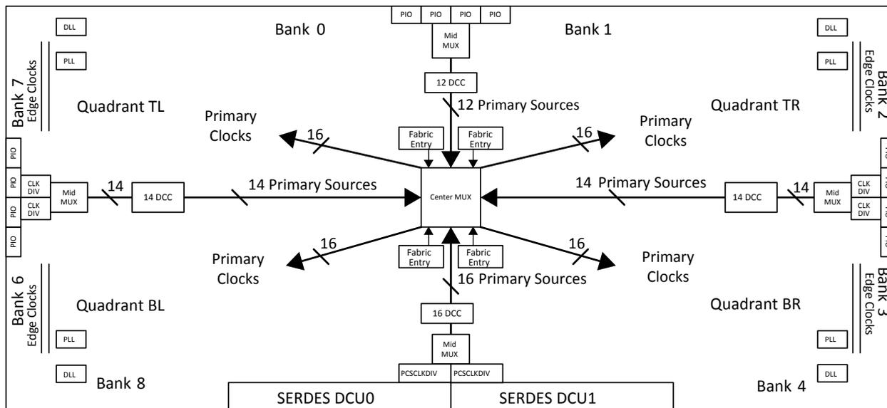
Figure 2.6. LFE5UM/LFE5UM5G-85 Clocking
