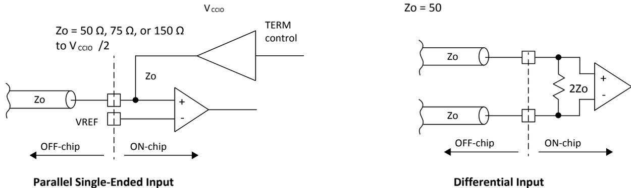
Figure 2.26. On-Chip Termination
