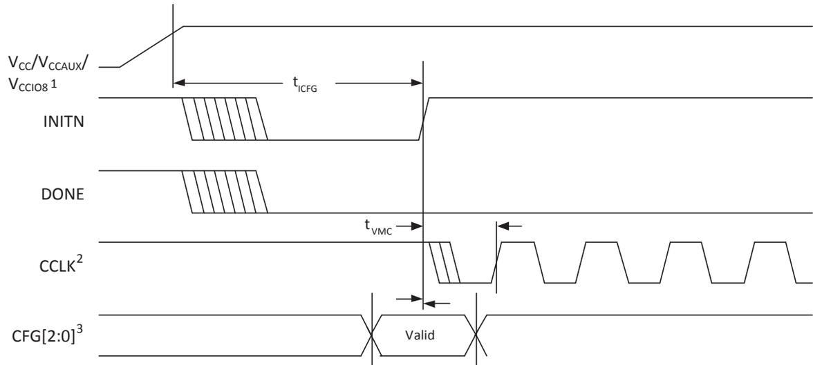
1. Time taken from V<sub>CC</sub>, V<sub>CCAUX</sub> or V<sub>CCIO8</sub>, whichever is the last to cross the POR trip point.
