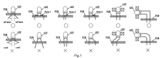
" $\bigcirc$ " Correct mounting method " $\times$ " Incorrect mounting method
