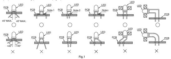
"( )" Correct mounting method "  $\times$  " Incorrect mounting method
