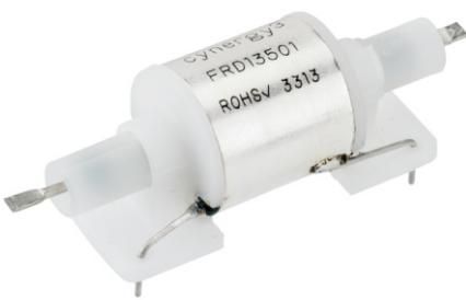
A complete RF screen around the coil assembly for a low loss transmission path, results in better carry current at elevated temperatures for this open frame series. An anti-corona sleeve is tted around the reed switch for improved RF voltage isolation. This type is widely used in HF Antenna Tuning Unit (ATU) applications.
