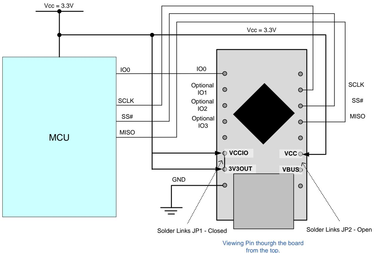
**Figure 5.5 – USB Self Powered 3.3V Logic Drive**
