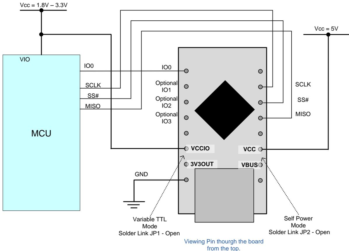
**Figure 5.2 – Self-Powered Configuration**
