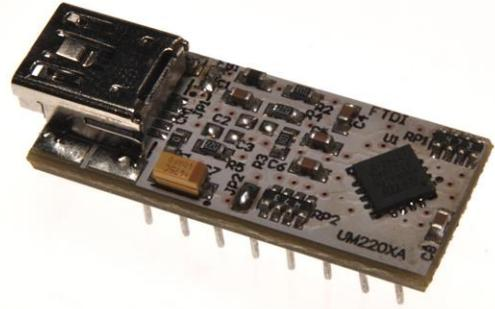
*UMFT220XA is a USB to 4-bit SPI/FT1248 DIP module with a 0.3" row pitch.*
