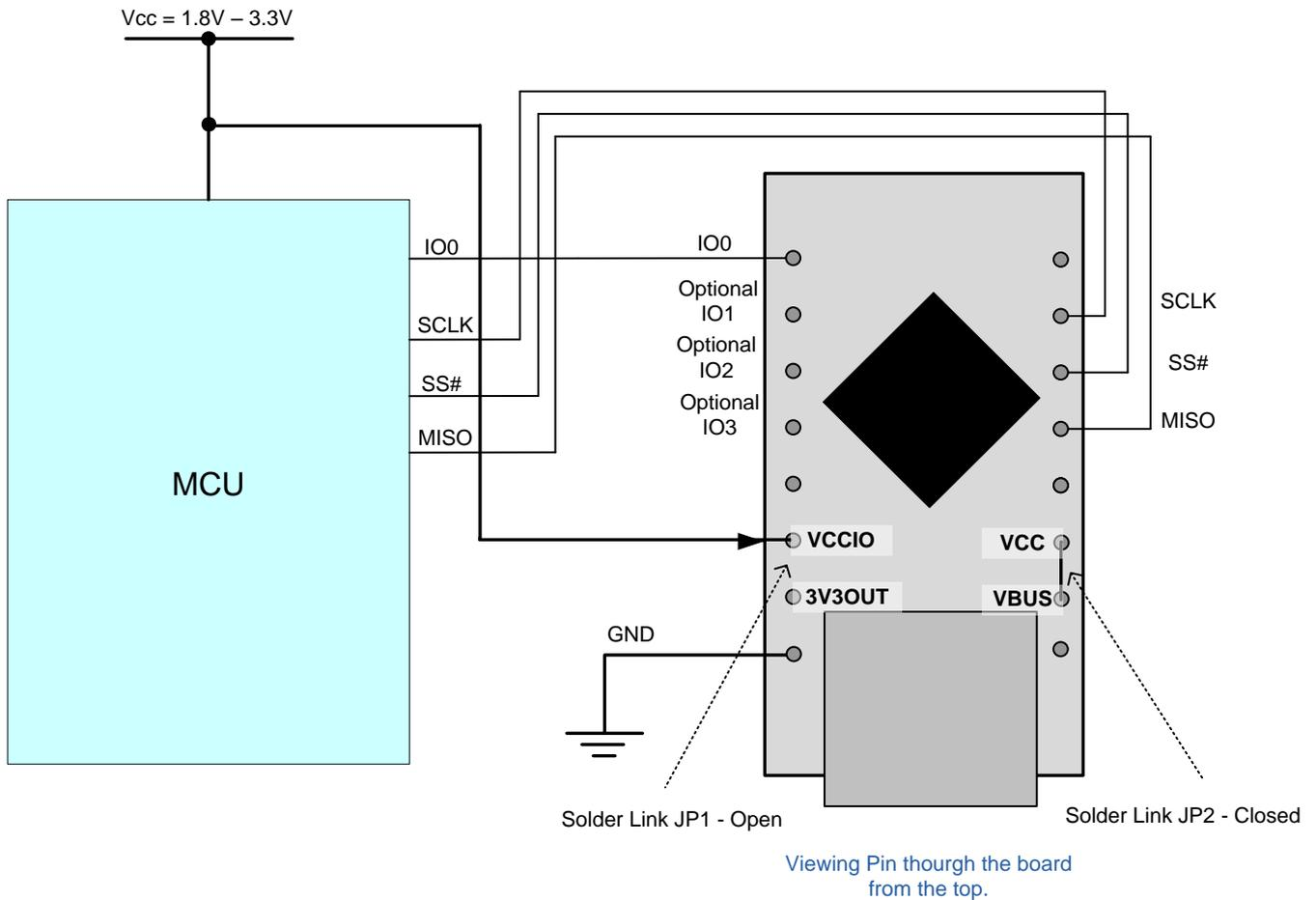
**Figure 5.4 – USB Bus Powered 3.3V Logic Drive**
