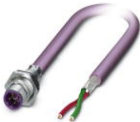
Bus system flush-type plug, PROFIBUS, 2-pos., M12, shielded, B-coded, rear/screw mounting with M16 thread, with 2 m bus cable, 2 x 0.25 mm 2
