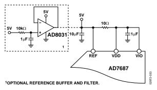
Figure 33. Example of Application Circuit
