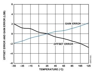
Figure 22. Offset Error and Gain Error vs. Temperature
