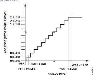
Figure 25. ADC Ideal Transfer Function
