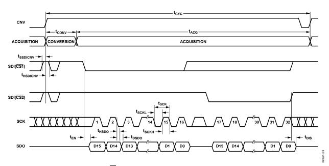
Figure 39. CS Mode, 4-Wire Without BUSY Indicator Serial Interface Timing
