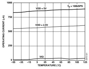
Figure 21. Operating Current vs. Temperature
