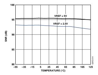
Figure 14. SNR vs. Temperature
