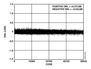
Figure 9. Differential Nonlinearity vs. Code
