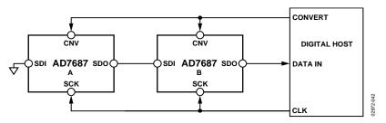
Figure 42. Chain Mode Without BUSY Indicator Connection Diagram
