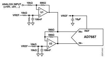
Figure 30. Single-Ended-to-Differential Driver Circuit
