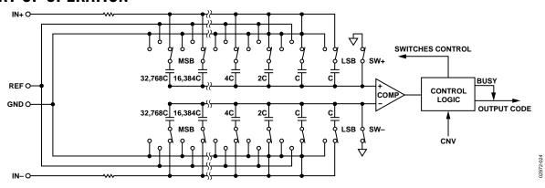
Figure 24. ADC Simplified Schematic
