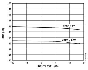
Figure 18. SNR vs. Input Level
