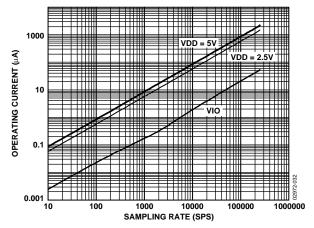
Figure 32. Operating Currents vs. Sampling Rate
