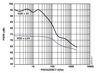
Figure 31. PSRR vs. Frequency
