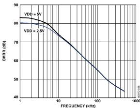
Figure 28. Analog Input CMRR vs. Frequency
