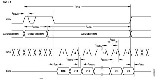
Figure 35. CS Mode, 3-Wire Without BUSY Indicator Serial Interface Timing (SDI High)
