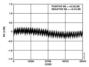
Figure 6. Integral Nonlinearity vs. Code
