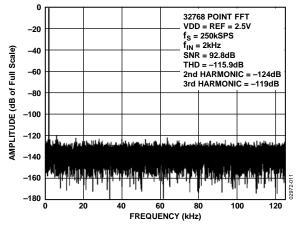
Figure 11. FFT Plot, VDD = REF = 2.5 V
