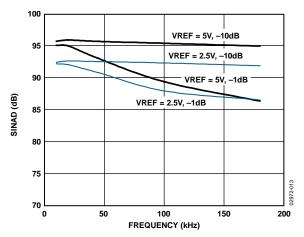
Figure 13. SINAD vs. Frequency
