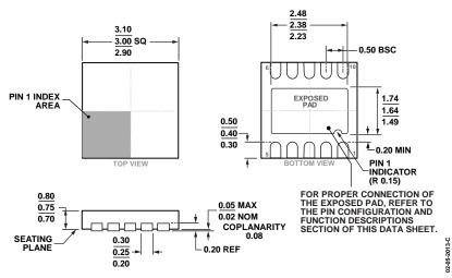
Figure 49. 10-Lead Lead Frame Chip Scale Package [LFCSP\_WD] 3 mm × 3 mm Body, Very Very Thin, Dual Lead (CP-10-9) Dimensions shown in millimeters
