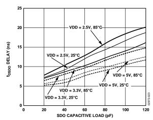
Figure 23. t<sub>DSDO</sub> Delay vs. Capacitance Load and Supply
