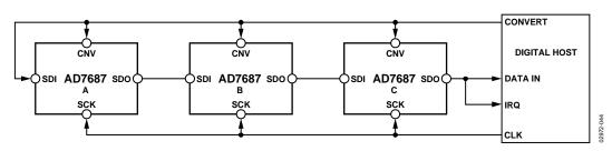
Figure 44. Chain Mode with BUSY Indicator Connection Diagram
