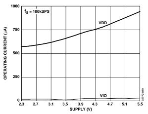
Figure 19. Operating Current vs. Supply
