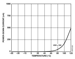
Figure 20. Power-Down Current vs. Temperature
