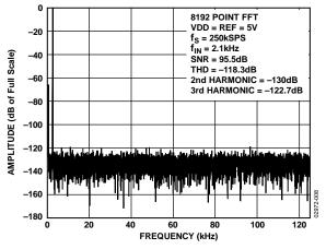
Figure 8. FFT Plot, VDD = REF = 5 V
