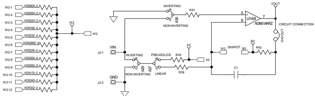
Figure 14. Schematic of Multiboard RDAC1 Circuits
