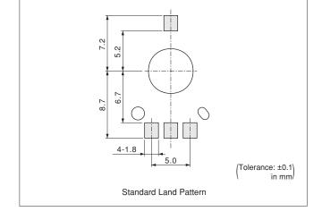
This product has two #2 terminals, at positions A and B to ensure flexibility of mounting on the board to cope with various wiring layouts.
